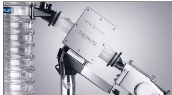
Metal check dust-tight connectivity
