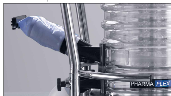
Fail safe air inlet
