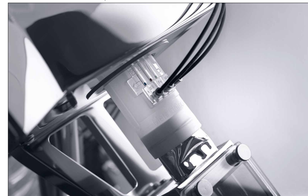
Optional Auto-Check for metal detector
