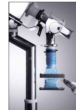
The liner film retracts in the clips when cutting
