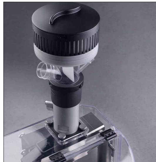
Dust-Tight tablet transfer
