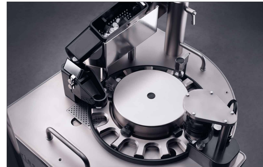
4-parameter IPC tester (weight - thickness - diameter - hardness)
